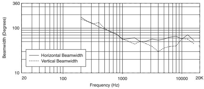
Measurements obtained in bi-amplified crossover mode.
