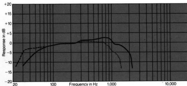
Frequency response contour of the 2240H/G taken in a hemispherical free-field environment, a closed box of 280 l (10 ft³) internal volume enclosing the rear of the driver. Measured response of a typical production unit, including all peaks and dips, does not deviate more than 2 dB from the above curve. The dashed curve represents the response from a 320 cm² (50 in²) port with a 20 cm (8 in) long duct tuning this enclosure to 30 Hz.
