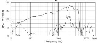
Measurements taken with an input of 15.5 V @ 1 meter (30 watts at 8 ohms). Distortion levels shown have been raised by 20 dB. The dashed line shows 2nd harmonic and the dotted line shows the 3rd harmonic. Note the lack of 3rd harmonic at high frequencies.
