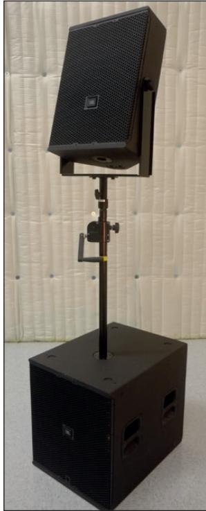
Ensure that the pole cup adapter is placed squarely on top of the mounting flange on the pole and that the –UB is tightened securely to the speaker. Failure to properly tighten the –UB to the speaker before attaching to the mounting pole could lead to an unsafe shift of the speaker or bracket.
