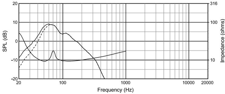
Control SB210 frequency response, (1W, 1m) at two-boundary junction ( $\pi$  loading, dotted line) and at three-boundary junction ( $\pi/2$  loading, solid) with recommended band-limiting filters (30 Hz high-pass 2nd order Butterworth, and 120 Hz low-pass 2nd order Butterworth).
