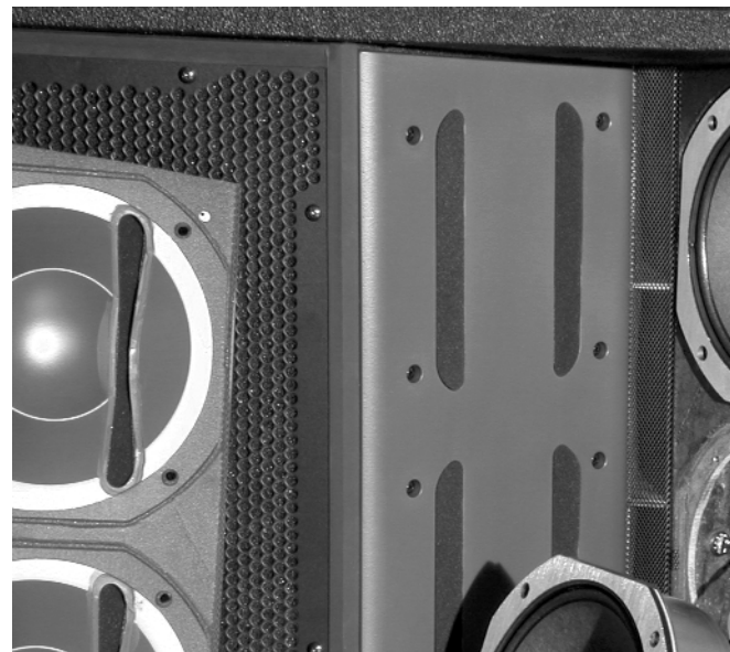
Open mid-range next to the WaveForm gap. Left shows the reverse of the 8" cover plate with affixed wave-guide and exit gaps for 8" speakers.
