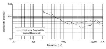
Measurements obtained in bi-amplified crossover mode
