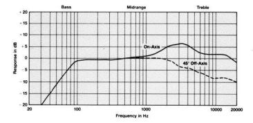
Frequency response contour of the 8140H taken in a hemispherical free-field environment. Measured response of a typical production unit, including all peaks and dips, does not deviate more than 4 dB from the above curve. Additional acoustic loading will further extend bass response.
