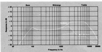
Frequency response contour of the 8120H taken in a hemispherical free-field environment. Measured response of a typical production unit, including all peaks and dips, does not deviate more than 4 dB from the above curve. Additional acoustic loading will further extend bass response.
