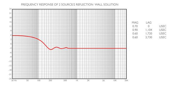
The second solution shown above includes two sources and two reflections. The lag times are achievable if one source is on the face of the loudspeaker and the second is on the rear of the loudspeaker. This solution has 9dB differential between coherency and incoherent summation, which could be usefulin some designs.
