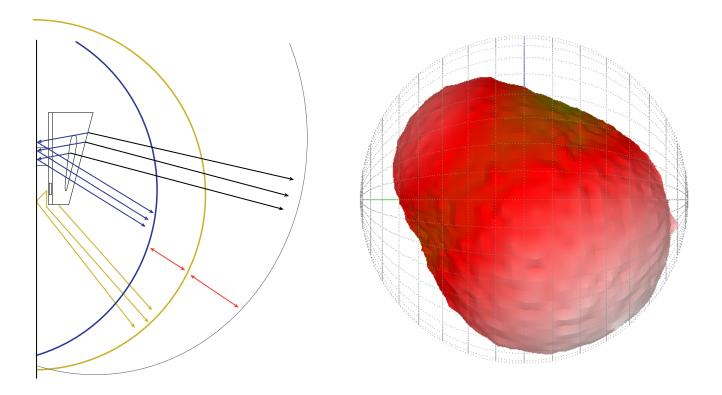
Further evidence of the two source arrangement within the 9350 is the radiation pattern of the loudspeaker shown above. The downward tilt in the pattern is not possible with one omnidirectional source. The radiation pattern is a result of the combination of sources presenting two wave fronts which sum together on the downward angles.
