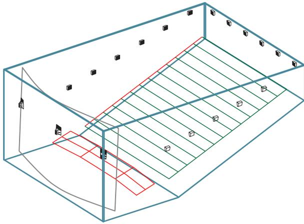
The importance of loudspeaker coverage in cinema is largely misunderstood. Despite often being described vaguely with specifications like “90x40,” it actually means how well loudspeakers interface or “uniformly map” with the audience.
