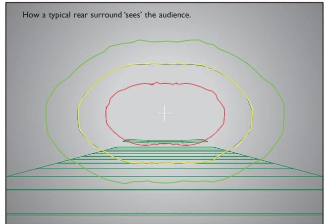
The resulting coverage map of a 7.1 rear surround array is shown on the bottom left. It has a severe rearward bias and a 7dB differential between the front seats and rear seats. In this example, the front half of the theater receives no intelligible rear content. Also, there is a 4dB differential between the rear row and calibration row. Evaluating the +/-1dB channel balance for all loudspeakers is now restricted to the box shown, which represents approximately a mere 7% of the audience!
