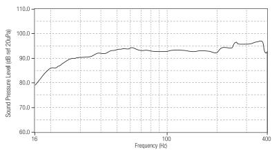
S2S-EX Subwoofer System, 1 meter @ 2.83v, 4 pi anechoic measurement
