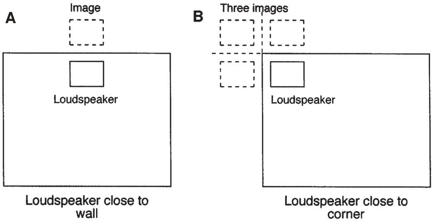
Figure 4. Loudspeaker boundary conditions. Against a wall (A); in a corner (B).
