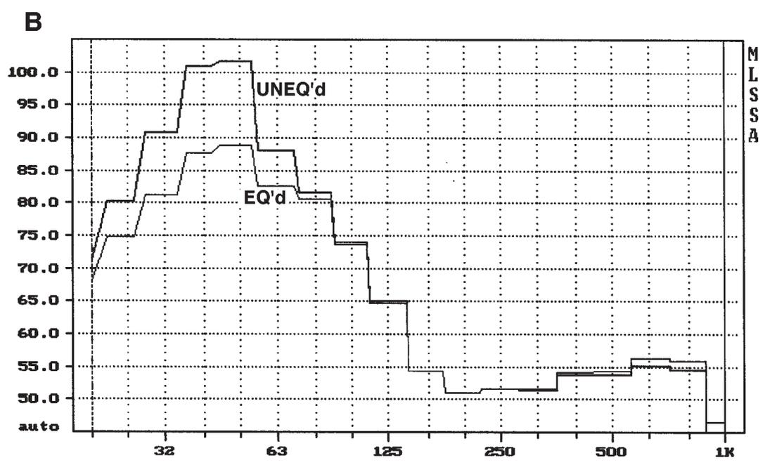
Figure 11. Same setup as before, but viewed with one-third octave analyzer (A); equalized with one-third octave equalization (B).
