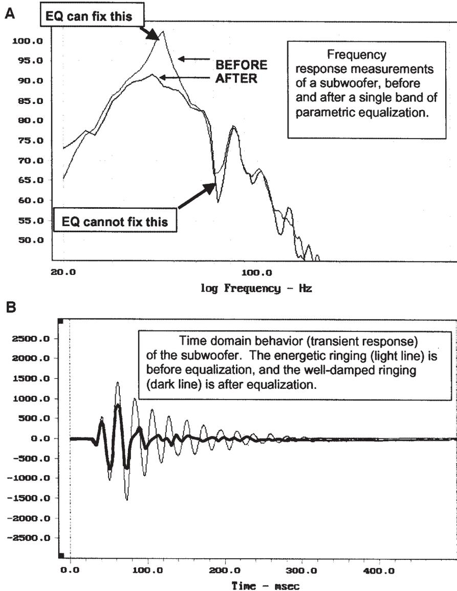
Figure 10. MLSSA measurements of a typical RMC equalization. Frequency response (A); time domain response (B).
