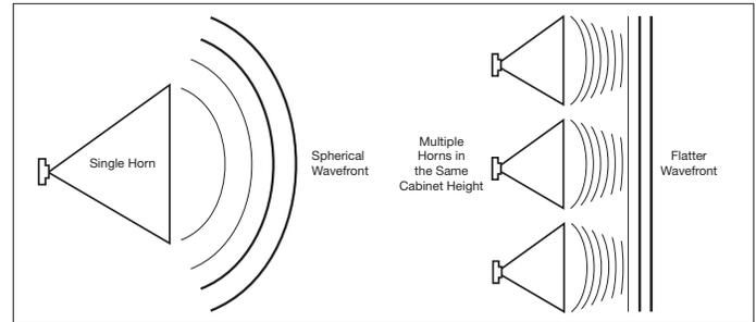
Spherical wavefronts tend to cause interference with adjacent loudspeakers. One common method for “flattening” the wavefront projecting from a vertical line array loudspeaker is to use multiple smaller horns instead of a single horn.
