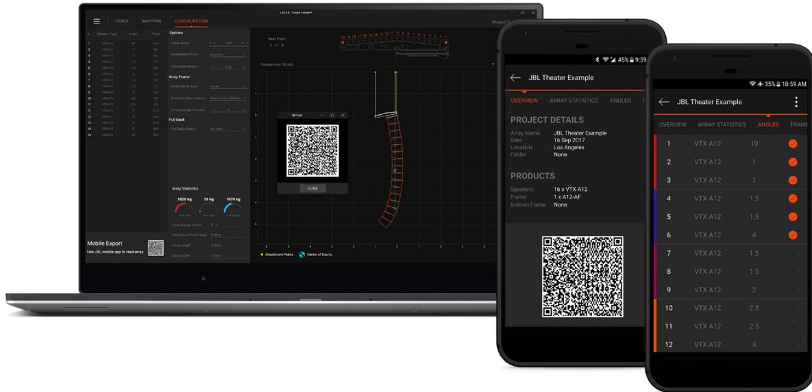
Once the system designer or lead tech computes the angles for each hang in LAC-3, every member of the crew can get the correct information for angles, attachment points, trim height, etc., either by scanning the QR code from LAC-3 directly with their device, or getting the data from a copy shared on another user's device. When all users onsite have the configuration data, arrays can be deployed quickly and efficiently.
