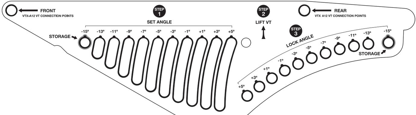
The Angle Selection mechanism settings correspond to the site angle of the VTX A12 enclosure connected to the GND (the bottom speaker of the array). For example, if -15° is selected on the GND, the bottom speaker of the array will point down at a 15-degree angle. If +5° is selected, the bottom speaker will point up at a 5-degree angle. These numbers are not related to the top enclosure of the array, and LAC-3 should be used to determine the overall angle of the ground stack.
