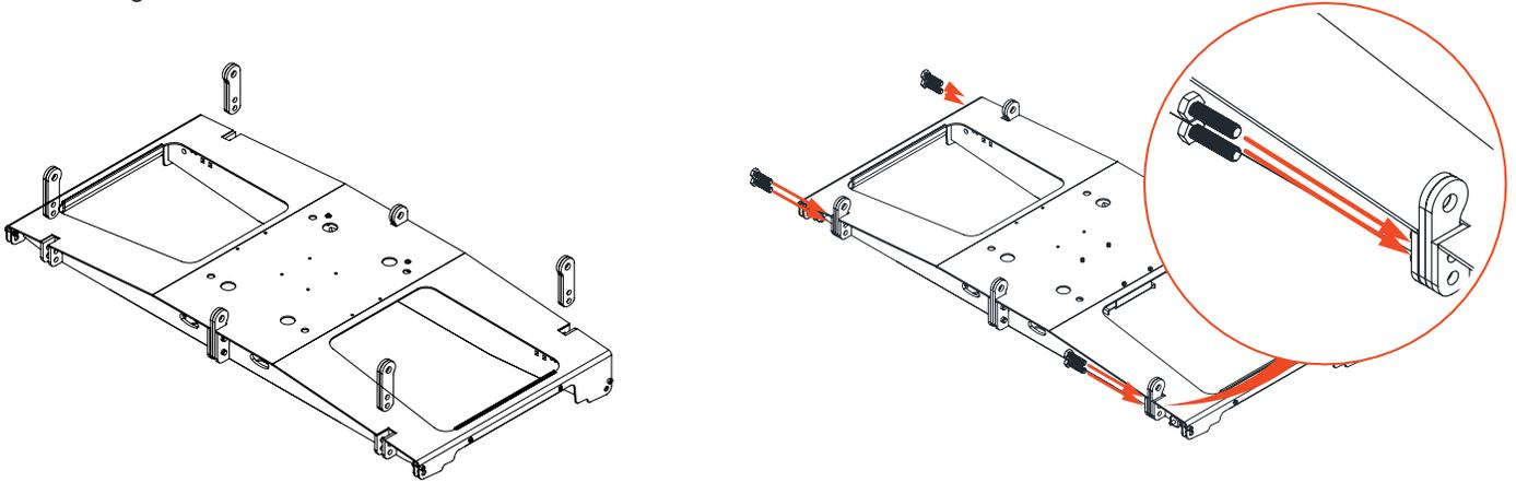
To attach two Extension Bars side-by-side, follow the instructions from section 8.3 Attaching the Extension Bar, mounting the Extension Bars to the tabs at the left and right Array Frame attachment locations.
