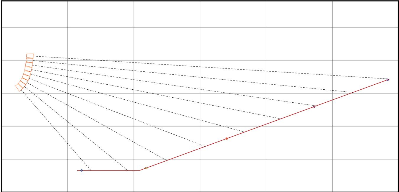
The venue geometry below calls for an array with its CoG perfectly lined up with the rear suspension point of the top A12 enclosure (LAC - Example 4). The flexibility of an Array Frame combined with an Extension Bar is not needed here, and a Suspension Bar can be used instead of an Array Frame (LAC - Example 5).
