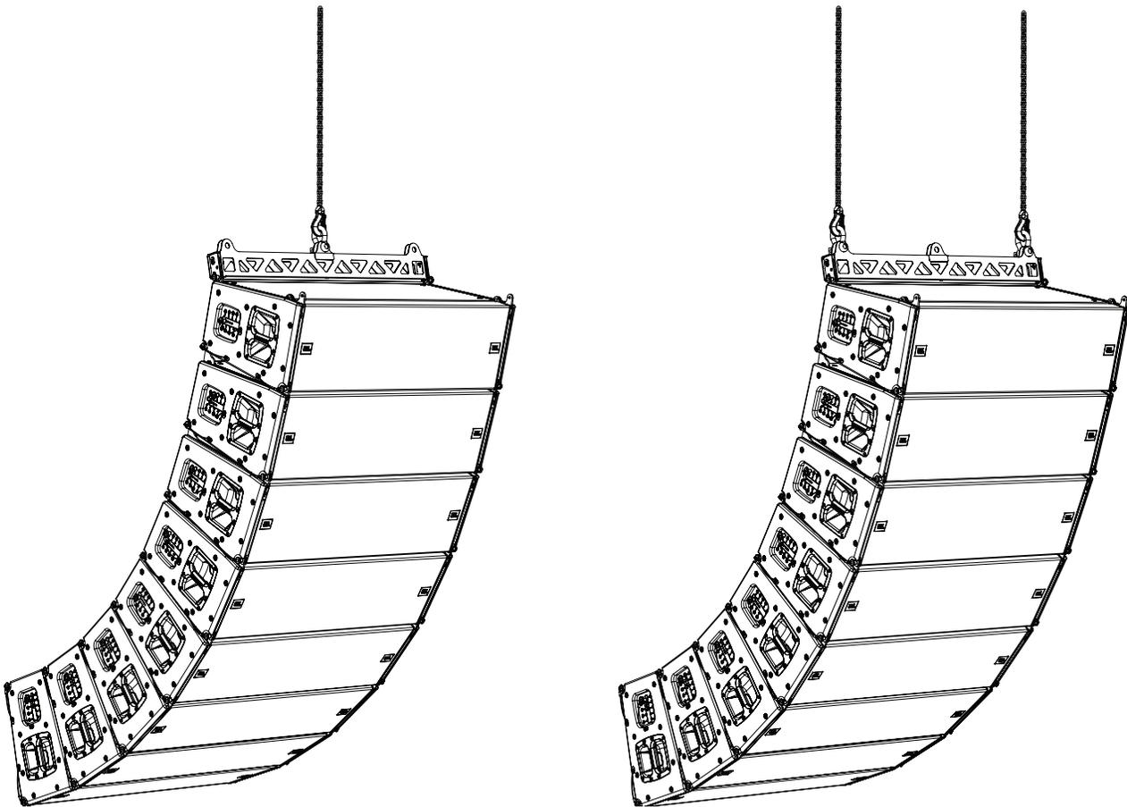
This configuration also supports side-by-side attachment for suspension hoists on the SB used as a top frame.
