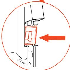
**NOTE:** The red Angle Lock levers are used to secure the angle position and prevent the cabinets from taking a different angle when cabinets are deployed in an array. The red Angle Lock lever is not load-bearing, and the system is safe even if they are accidentally left in the unlocked position.
