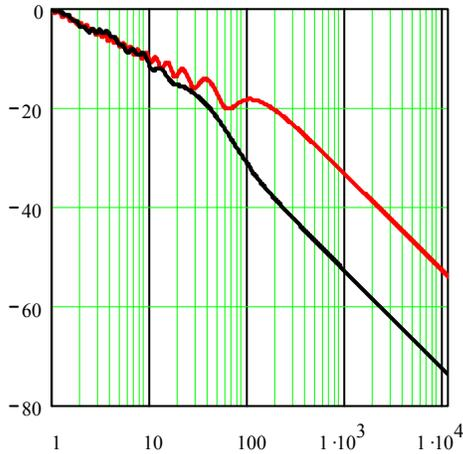
**Figure 10: On-axis pressure response of an arc source and a straight line source at 2kHz. The line source has a length of 4 meters. The arc source is 30deg and a radius of 8 meters providing an equivalent total length of 4m.**
