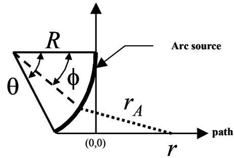
**Figure 9: Geometric construction of an arc source.**
