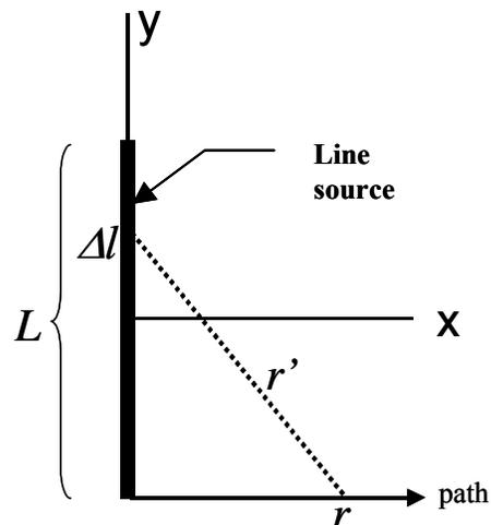
**Figure 5: Geometric construction to calculate the pressure response along a path originating at the endpoint.**
