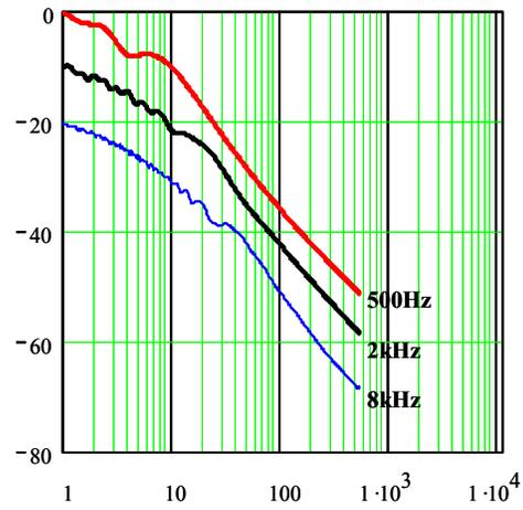
**Figure 12: On-axis pressure response of three arc sources at various frequencies where  $\theta = 60^\circ$  and  $R = 4m$ . The 2kHz and 8kHz curves are offset by 10 and 20 dB respectively.**
