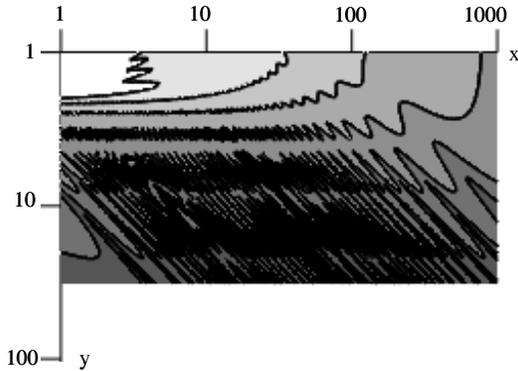
**Figure 8: Pressure field of a 4-m line source at 8kHz. The source is located in the upper left corner (not shown) facing to the right. The x-axis in the figure is coincident with a path, normal to the source, starting at its midpoint.**
