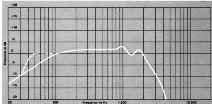
The solid line depicts the frequency response of Model 2203H in a closed box of 280 L (10 ft<sup>3</sup>) volume. The response of a typical production unit, including all peaks and dips, does not deviate more than 2 dB from this curve. The dotted curve represents a typical application of the loudspeaker, mounted in 57 L (2 ft<sup>3</sup>) with a port tuning the enclosure to 28 Hz.
