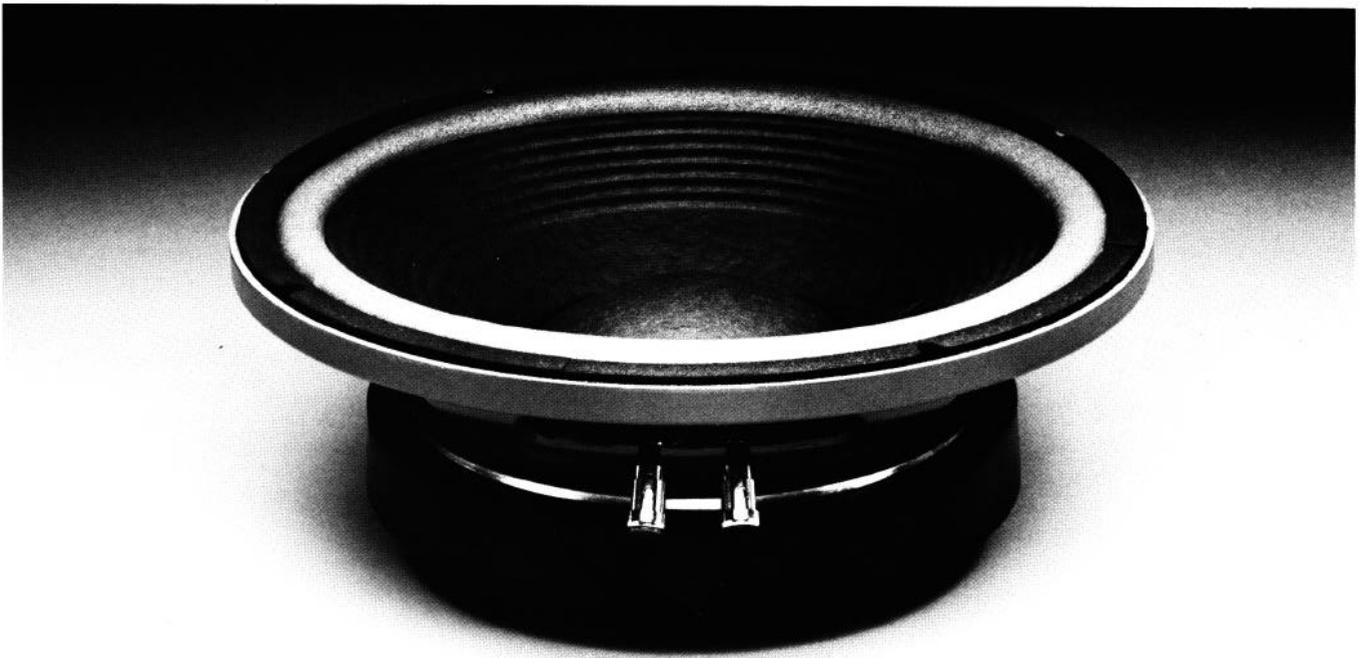
The Model 2203H is a 300 mm (12 in) low frequency loudspeaker that delivers the accuracy and extended bandwidth of the larger Model 2231H. Flat, deep bass ( $\pm 2$  dB, 40 Hz to 800 Hz, measured on axis) and excellent transient response favor its use in systems such as studio monitors, where small size and maximum bandwidth are of critical importance.
