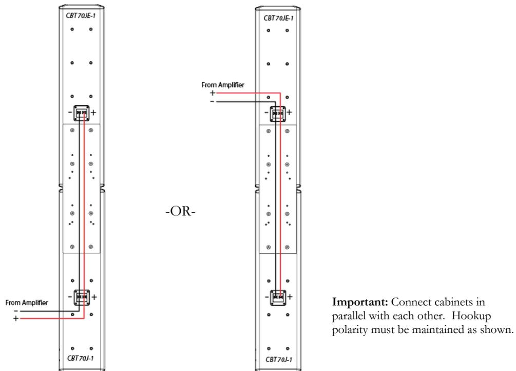
Stated from the amplifier side, wire from the amplifier to one of the cabinets (it doesn't matter which cabinet) and use a jumper speaker wire (“+” and “-”) to run the plus and minus in parallel to the other cabinet.
