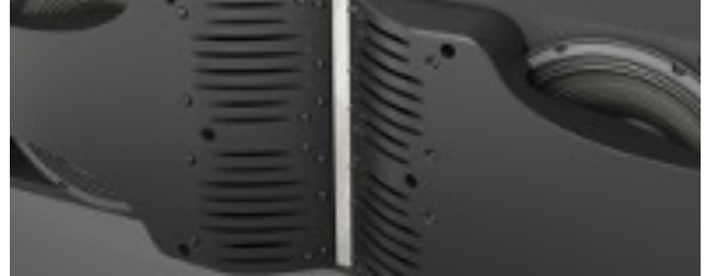
ACOUSTIC LOADING APERTURE OVER EON 600 LF DRIVER IMPROVES DIRECTIVITY (SHOWN WITH INCLUDED GRILLE REMOVED)
