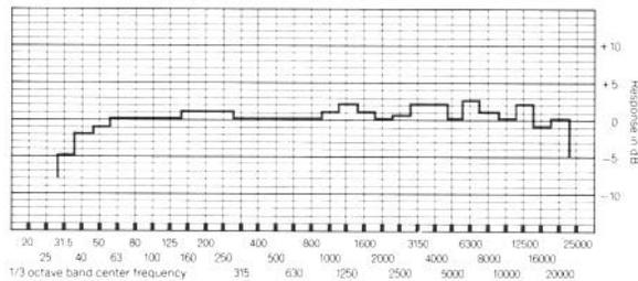
Frequency response of the 4315 taken with 1/3-octave band pink noise. Measured response contour of a typical system averaged through an inclusive arc of 80° in the horizontal and 60° in the vertical planes does not deviate more than 2 dB from the above curve.
