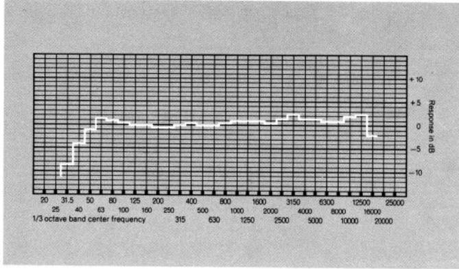
Frequency response of the 4301BE taken with 1/3-octave band pink noise. Measured response of a typical production system averaged through an inclusive arc of 30° vertically and horizontally does not deviate more than 3 dB from the above curve.
