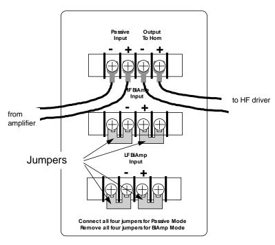
To bypass the internal passive crossover network **for bi-amplified operation**, remove all four jumpers and connect as shown:
