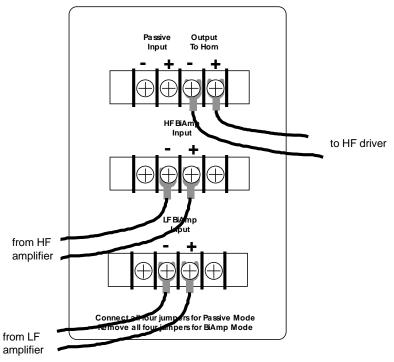
Note that in both passive and bi-amplified mode, the same HF driver cable connection is made.
