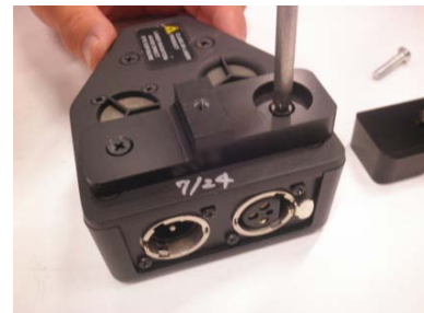
Remove the mount tab including quick release pin (QRP) and lanyard
