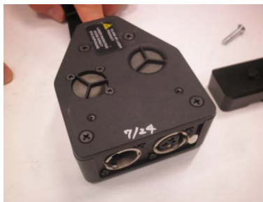
Remove mount tab base, rotate 180 degrees and re-install
