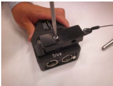
Remove the mount tab including quick release pin (QRP) and lanyard
