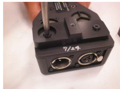
Remove mount tab base, rotate 180 degrees and re-install
