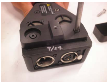
Rotate mount tab / QRP / lanyard assembly 180 degrees, re-attach to mount tab base
