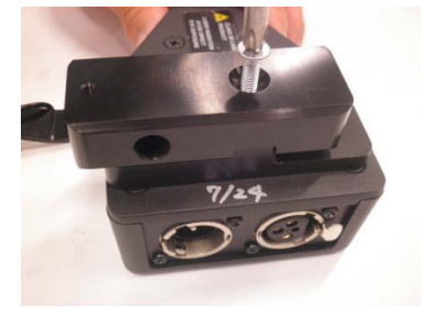
Rotate mount tab / QRP / lanyard assembly 180 degrees, re-attach to mount tab base
