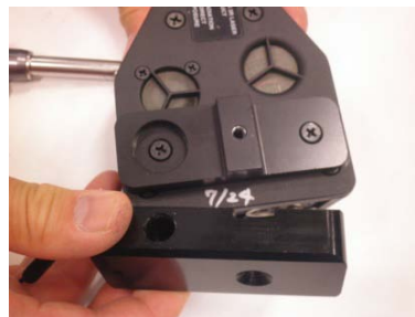
Rotate mount tab / QRP / lanyard assembly 180 degrees, re-attach to mount tab base
