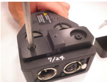
Remove mount tab base, rotate 180 degrees and re-install
