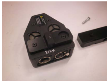
Remove the mount tab including quick release pin (QRP) and lanyard
