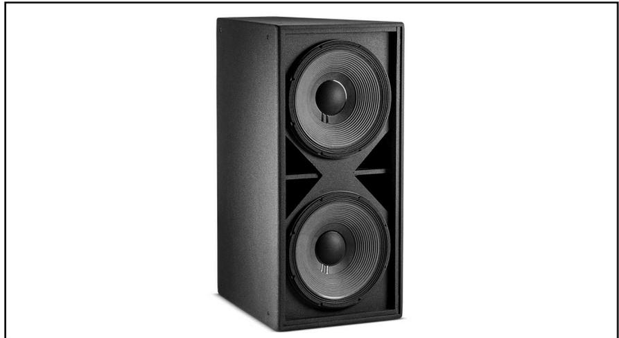
The PD5125 is a high power low frequency loudspeaker comprised of two 380 mm (15 in) VGC™ Vented Gap Cooled low frequency drivers in a front-loaded, vented configuration. The trapezoidal cabinet is fitted with M10 threaded suspension points.
