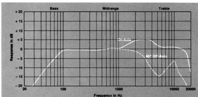
Frequency response contour of the 8130H taken in a hemispherical free-field environment. Measured response of a typical production unit, including all peaks and dips, does not deviate more than 4 dB from the above curve. Additional acoustic loading will further extend bass response.
