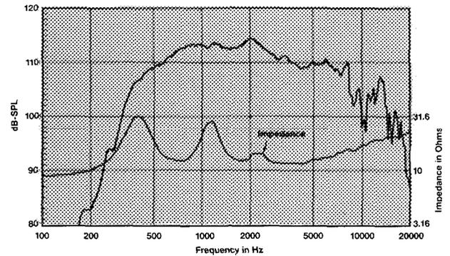
Frequency response of the 2447H coupled to a JBL 2352 Bi-Radial® Horn, measured on-axis at a distance of 1 meter with a 1 watt (2.83 V RMS) input in a reflection free environment, with impedance vs. frequency curve.
