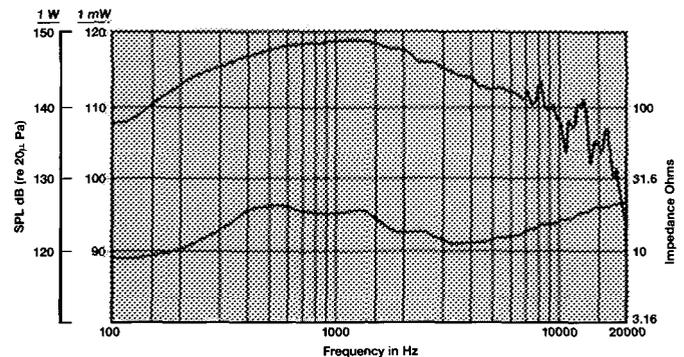
Frequency response and impedance modulus of model 2447H coupled to a 38 mm (1½ in) diameter terminated plane wave tube. This is the power response of the transducer, and is the frequency response that will be obtained on a true full range constant directivity horn design, such as JBL's 2350 series of Bi-Radial® horns.
