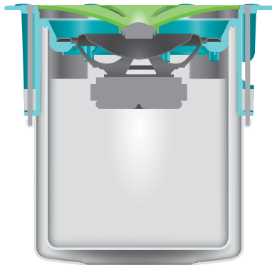
Fig. 2, JBL Control 445 Cutaway, Conical RBI™ design featuring two baffles.
